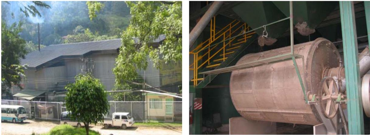
Fig. 3: Coffee drying, Coopeldos, Costa Rica, Installed capacity: 595 kW<sub>th</sub> (850 m<sup>2</sup> Solar Wall collector)
