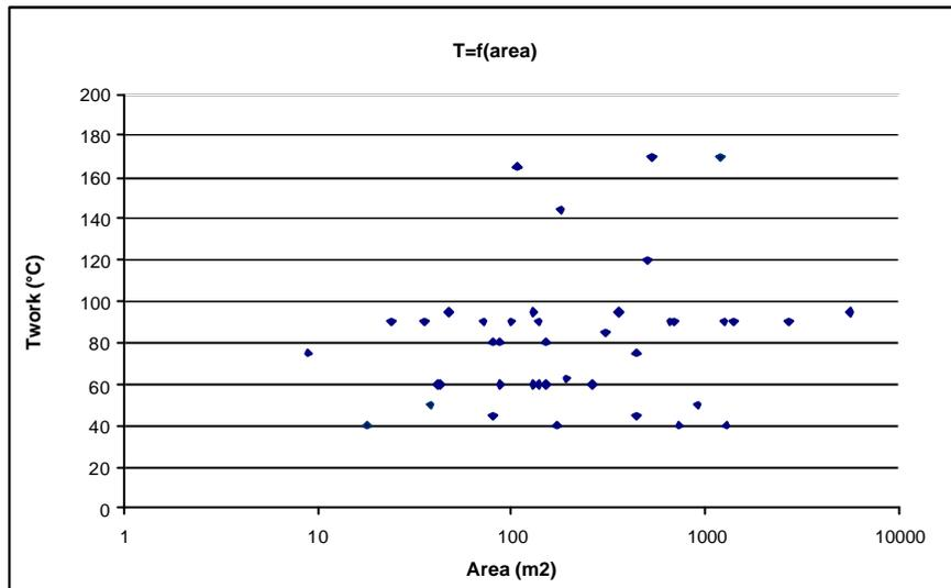
Figure 3: Solar plants documented by Task 33/IV: Correlation of working temperature vs. solar field size. State: April 2004.
