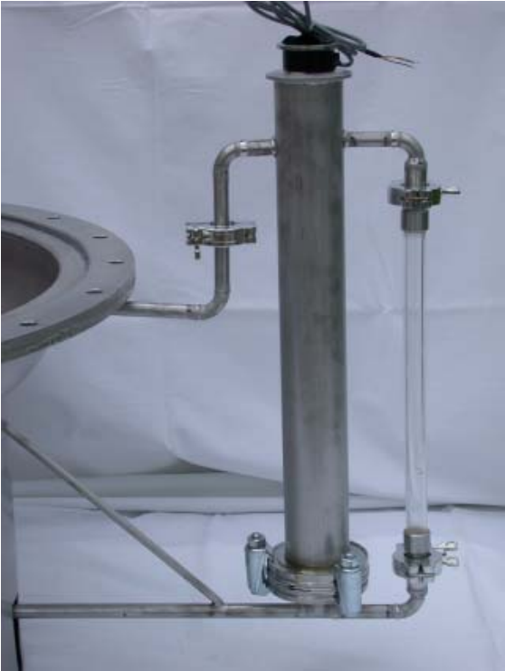
Figure 5: Water level measurement (right hand side: viewing glass, middle: water level sensor)
