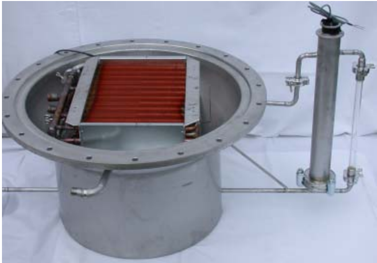
Figure 4: Lower part of the prototype module with evaporator/condenser heat exchanger
