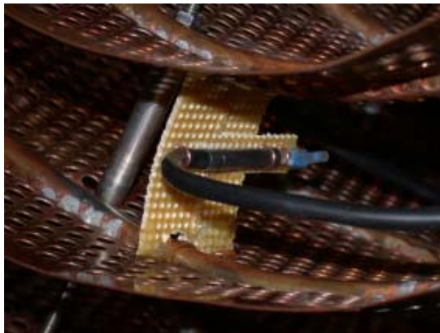
Figure 3: Mounting of temperature sensors in the silica gel packing
