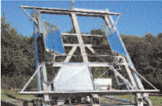
ABOVE Testing of two PTC 1000 modular parabolic trough collectors at DLR in Germany. In these tests the collectors are installed on a tilted testing platform so that the effect of end-losses are eliminated ABOVE RIGHT Solar-heated production hall and office building DOMA
